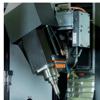
接触式对刀仪 Tool setting device contact
