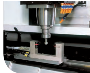
激光对刀仪 Laser tools setting device
