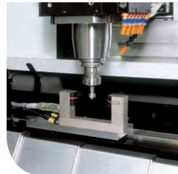
激光对刀仪 Laser tools setting device
