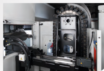
配有机械手的链条式刀库 Chain magazine with exchanging arm
