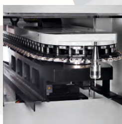
链条式刀库 Movable chain magazine
